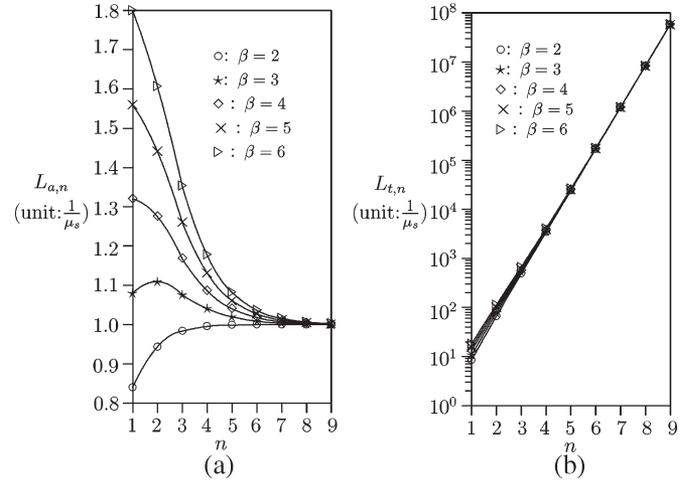
Fig. 4. Effects of  $n$  and  $\beta$  on  $L_{a,n}$  and  $L_{t,n}$  [ $\lambda_o = 10\mu_s$ ;  $\eta_a = (2/3)\mu_s$ ;  $v_a = 1/\eta_a^2$ ].
